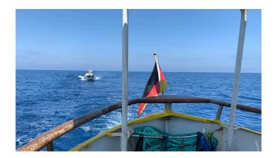
Maybe adjust the length of the ropes, so that there is the same power on both ropes. Adjust the towing-lines to equal length by tossing them ½ or 1 time around the bollard if needed.
